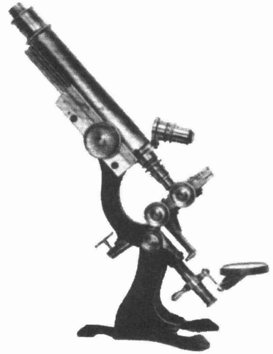
Typical appearance of early microscope, around 1870, manufactured in the US, the first with more than one objective.
